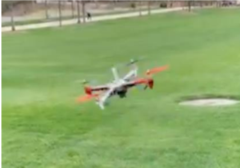
Figure 4. Unstable drone about to tip over
