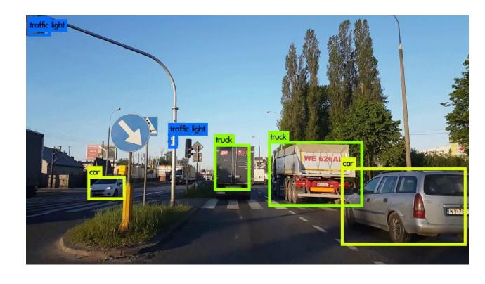
OpenCV algorithms used on the Jetson will detect and locate objects in the drone's reference frame.
