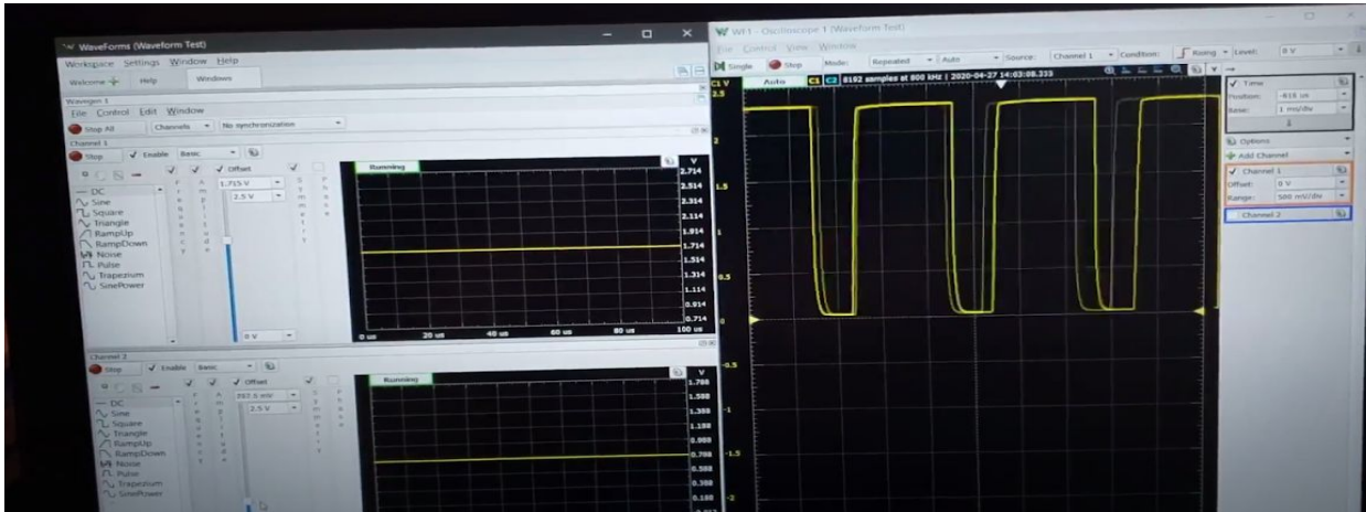
Figure 5-4. Oscillation of the Electronics for Music Applications Team’s VCO at V_{ref} = 1 V as V_{bp} and V_{bn} are varied. At this point, V_{bp} = 1.715 V and V_{bn} = 252.5 mV. The output appears to be a square wave.
