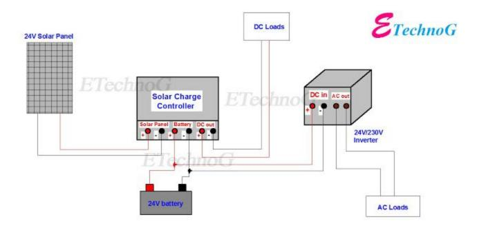
Figure 1. Diagram showing the interconnection between solar-panel and charging circuit [4].
