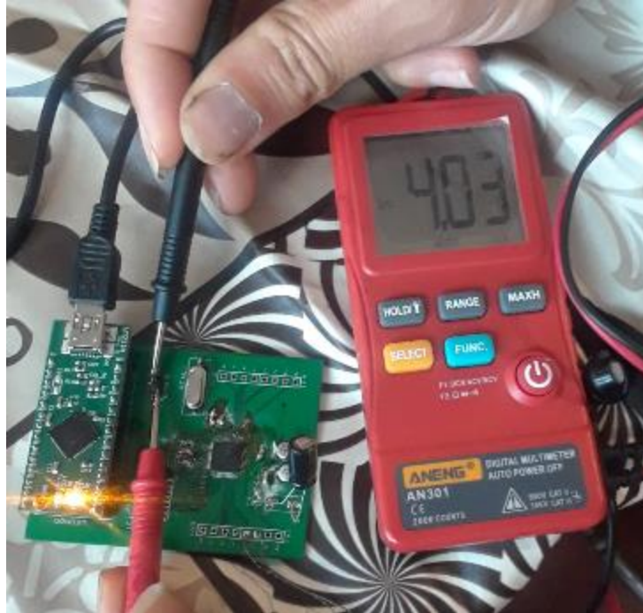
Fig. 1. This figure is the test of the power line to be sure that the board is being provided with power.
