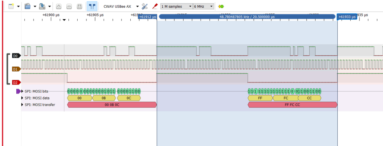
Fig. 8. Frequency of LRCLK doubling verified by logic analysis. The period changed from 41 μs to 20.5 μs.
