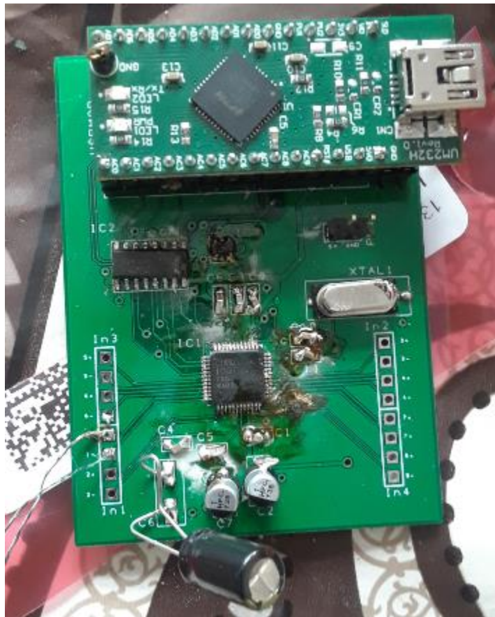
Fig. 4. Circuit assembled for first phase of testing. The extending cables are the stereo connector connection onto the surface.
