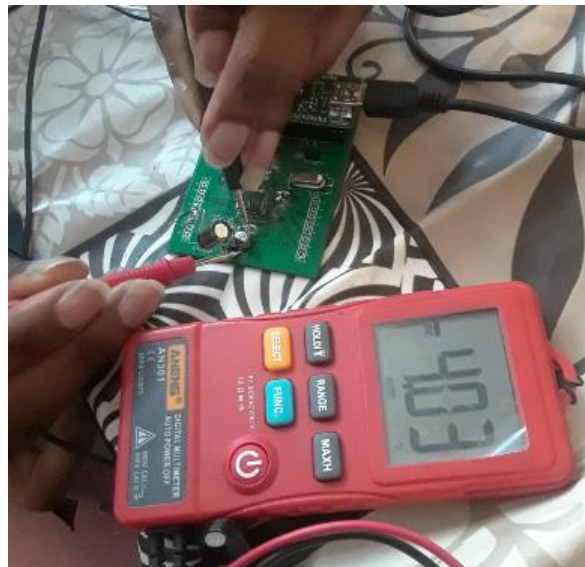
Fig. 2. Voltage across the capacitor matched that which was supplied as expected.
