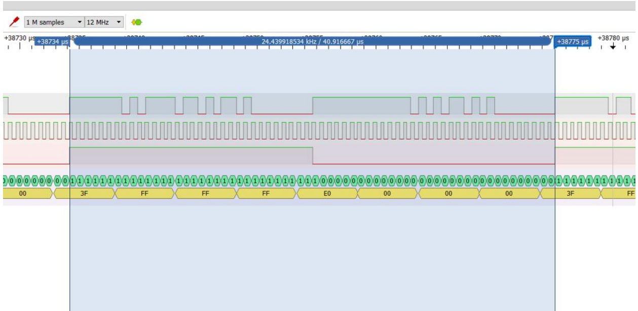
Fig. 9. Frequency of LRCLK used to be half that of figure 8. upon change by software and period used to be approximately 41 μs.
